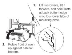
Insert a self-aligning screw through top center cabinet hole. Temporarily secure the oven by turning the screw at least two full turns after the threads have engaged. (It will be completely tightened later.) Be sure to keep power cord tight. Be careful not to pinch the cord, especially when mounting flush to bottom of cabinet.
