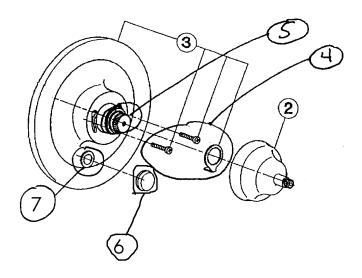
MOUNTING SCREWS+CAM+DIVERTER ASSEMBLY 2303-1210 MOUNTING SCREWS
