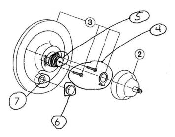
MOUNTING SCREWS+CAM+DIVERTER ASSEMBLY 2303-1210 MOUNTING SCREWS
