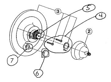
MOUNTING SCREWS+CAM+DIVERTER ASSEMBLY 2303-1210 MOUNTING SCREWS
