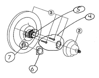
MOUNTING SCREWS+CAM+DIVERTER ASSEMBLY 2303-1210 MOUNTING SCREWS
