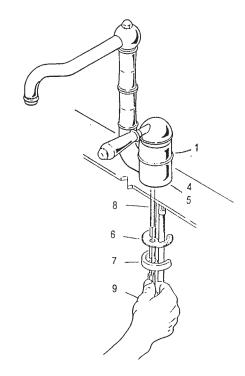
Under the sink, stack the half ring rubber gasket - 6, the half ring mouting plate - 7, then the mounting nut -9 onto the stud.
