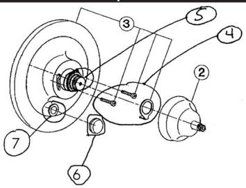
MOUNTING SCREWS+CAM+DIVERTER ASSEMBLY 2303-1210 MOUNTING SCREWS
