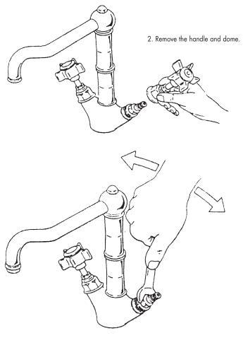
3. Remove the cartridge with a smooth jawed wrench or  $17\,\mathrm{mm}$  wrench
