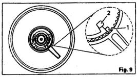
Place the lever handle onto the intermediate handle, lining up the handle stop (1) with the escutcheon stop post (2).
