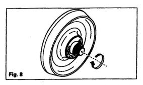
Rotate the intermediate handle clockwise until it stops, closing the valve.
