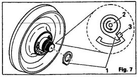
■ Place the handle position stop (1) over the splines on the intermediate handle (2) with the stop ring resting against the escutcheon stop post (3).
