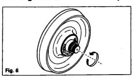
Rotate the intermediate handle counterclockwise until a desired and safe hot water temperature is reached (recommended maximum is 110 °F / 43.3 °C).
