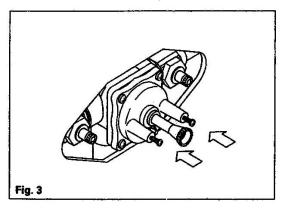
Install the two packaged escutcheon screws into the valve cover tappings. These screws allow for variation in wall thickness when mounting the escutcheon to the valve cover.
