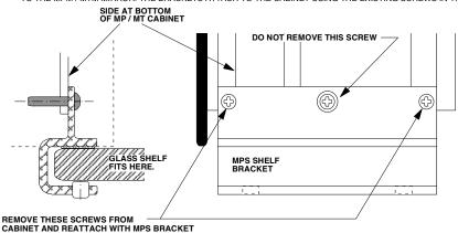
2. BE SURE THE OPEN SIDE OF THE BRACKET FACES THE MPM / MTM MIRROR. INSTALL THE CABINET, (LIGHT IF USED) AND SIDE KIT AS PER C ABOVE.
