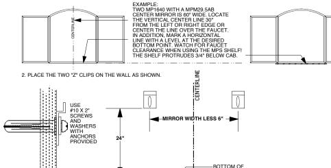
3. TEST FIT THE MIRROR. ADJUST CLIPS IF NECESSARY. WITH A PENCIL, MARK THE LEFT AND RIGHT EDGES OF THE MIRROR. REMOVE THE MIRROR WHILE INSTALLING THE CABINETS. BE CAREFUL NOT TO CHIP THE EDGES.
