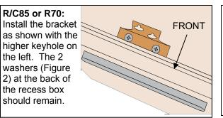
R/C85PLUS, R75LSe, R94LSe: Install the bracket FRONT as shown with the lower keyhole on the left. Remove the 2 washers (Figure 2) at the back of the recess box.
