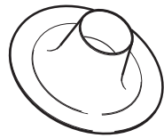
9 flat roof flashing
