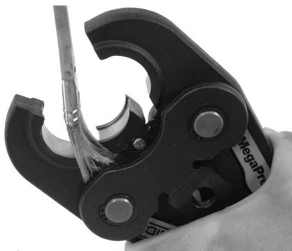
Figure 12 – Cleaning Segment Area of MegaPress Jaw
