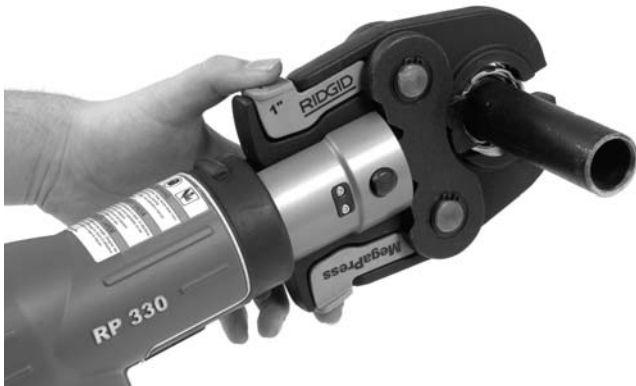
Figure 8 – Opening the MegaPress Jaw set and Placing Around Fitting
