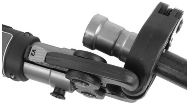
Figure 11B – Placing V2 Actuator Into MegaPress Ring Pockets At An Angle For Additional Clearance
