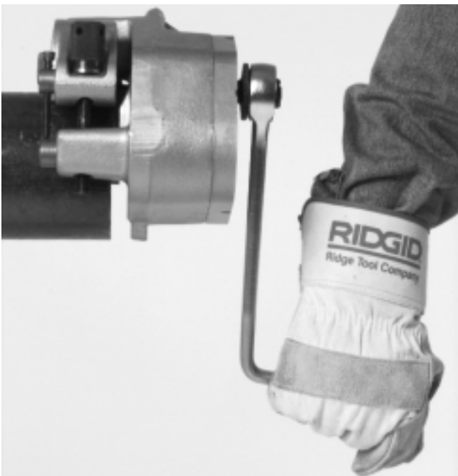
Figure 6 – Rainurage du tuyau
