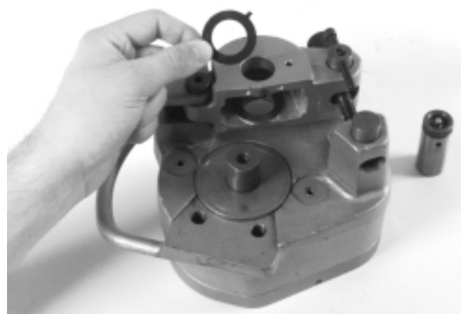
Figure 10 – Placement of Thrust Washer
