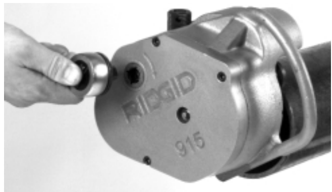
Figure 7 – Ratchet in Input Drive
