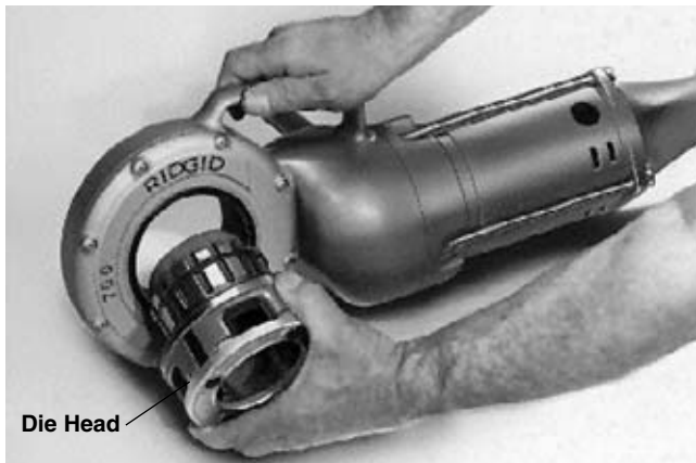
Figure 3 – Installing No. 12-R Drop Head Die Head
