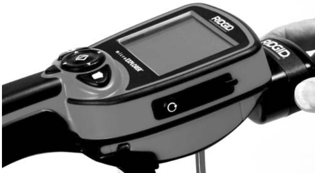
Figure 10 – Connecting the microEXPLORER Camera Monitor
