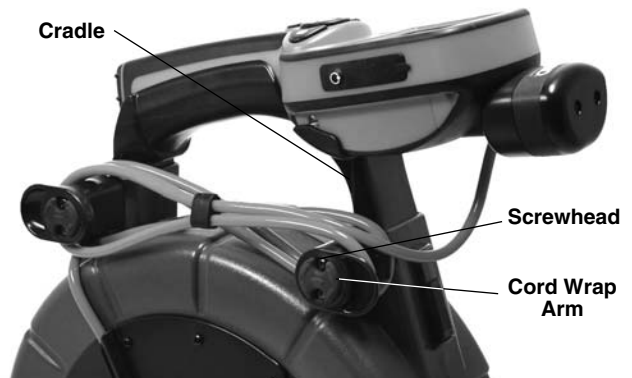
Figure 9 – Cradle Support and Cord-Wrap Arms
