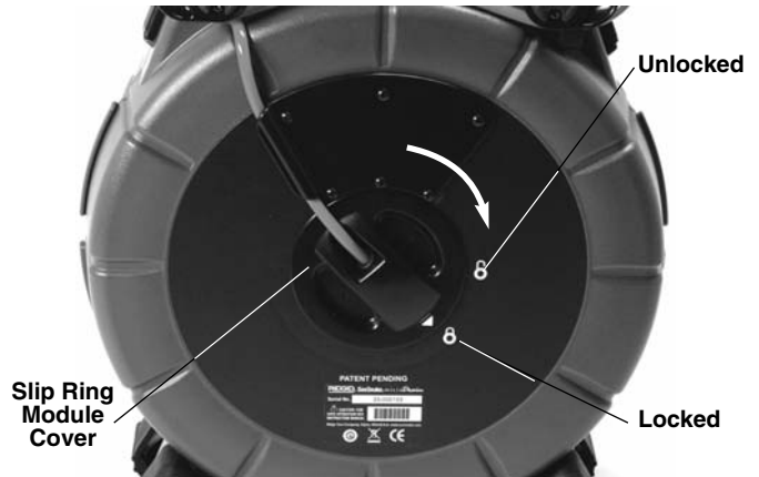
Figure 8 – Locking The Slip Ring Module Cover
