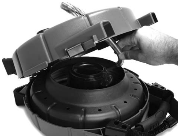
Figure 5 – Routing The Camera Head
