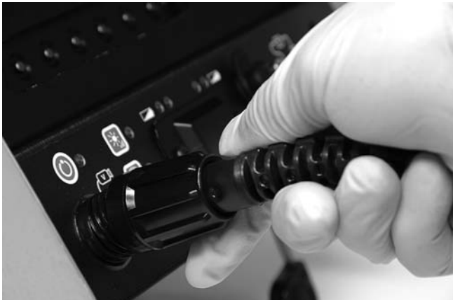
Figure 13 – Connecting To A SeeSnake CCU
