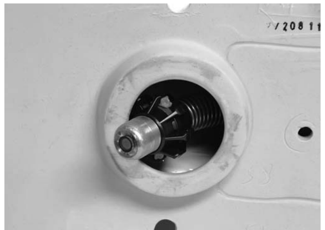
Figure 21 – Camera Head with Ball Guide in Turn
