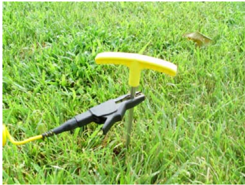
Figure 7: Attaching Lead to Ground Stake
