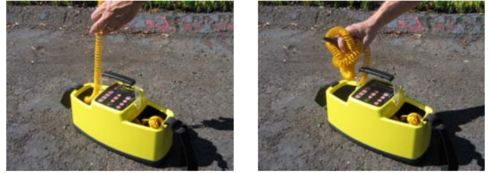
Figure 20: Storing Leads: Right Way and Wrong Way
