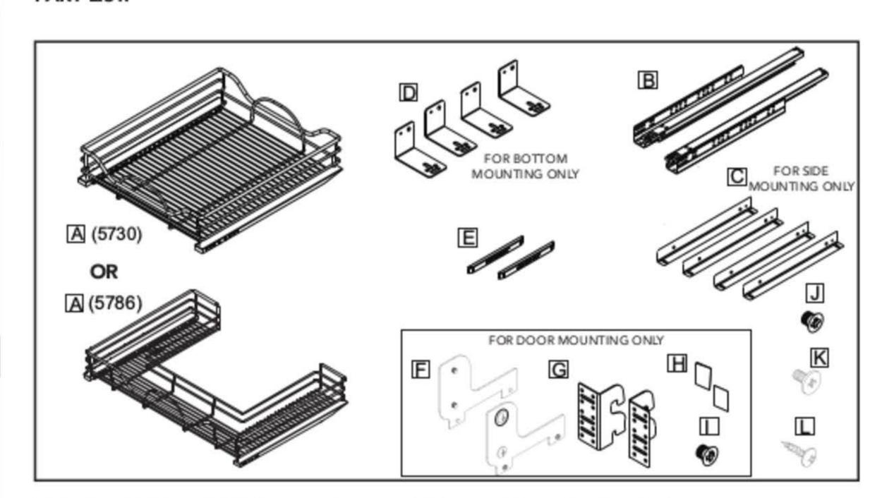
(A) Basket, (B) Slide, (C) Side mount bracket, (D) Bottom Mount bracket, (E) Logo cap, (F) Mounting bracket, (G) Door mounting bracket, (H) Double sided tape, (I) M4 x 6mm Machine screw, (J) M5 x 6mm Machine screw, (K) M5 x 10mm Flat Machine screw, (L) 5/32 x 18mm Wood Screw
