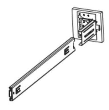
Step1: Install rear bracket to rear of slide.
