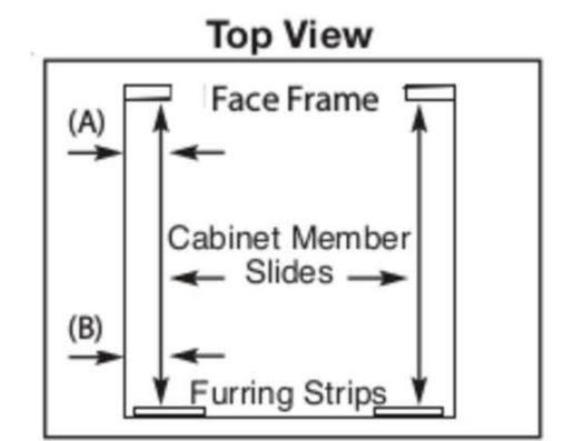
Step 5: Mount Rear Bracket. Extend the slide rear mounting bracket until it contacts the rear (Furring Strip). Bottom of slide should be(13½%-35 & 27Qt. 19"-50Qt.) from cabinet floor. Rear mounting bracket should be the same distance from the side cabinet wall at rear of slide as it is up front. Drive mounting screw in center horizontal slot of rear mounting bracket, tighten. Tighten screw in front bracket.
