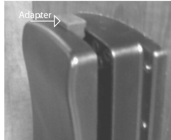
3. Push adapter into top front of unit until fully seated in PDCR slot.
