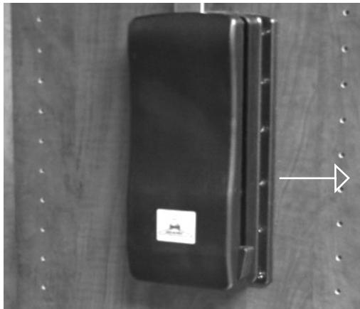
1. Install PDCR according to included instructions, ensure that unit is as close to front of closet panel as possible once installation is complete.
