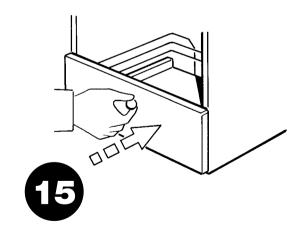
WITH SLIDES IN CLOSED POSITION, SET UNIT ON SLIDES AND PUSH IN AS FAR AS IT WILL GO. THIS WILL ENGAGE LOCK ON TO SLIDES.
