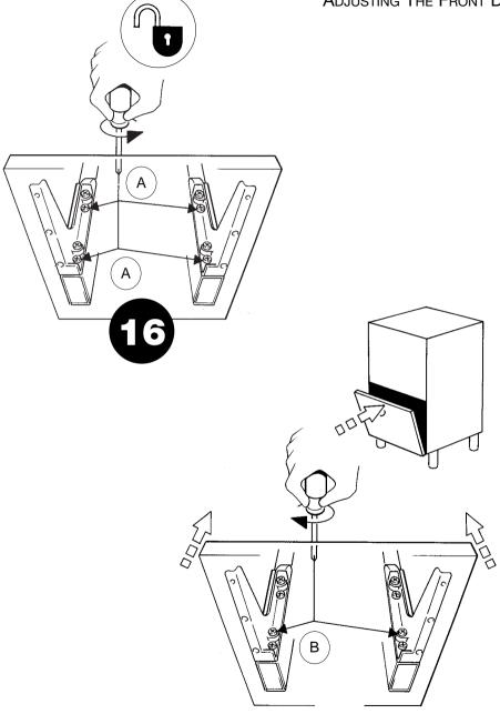
WHEREAS TO TILT TOP OF DOOR OUT, LOOSEN ATTACHMENT SCREWS (A), TIGH-TEN BACK ADJUSTMENT SCREWS (B)
