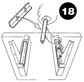
INSTALL SNAP ON COVER OVER ATTA-CHMENT AND ADJUSTMENT SCREWS. REMOVING THE UNIT
