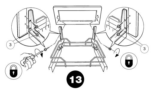
ATTACH BASKET WITH BRACKETS TO CABINET DOOR. BE SURE UNIT IS CENTERED SIDE TO SIDE AND AT THE PROPER HEIGHT TO ALLOW PROPER OVERHANG OF DOOR AT TOP AND BOTTOM.
