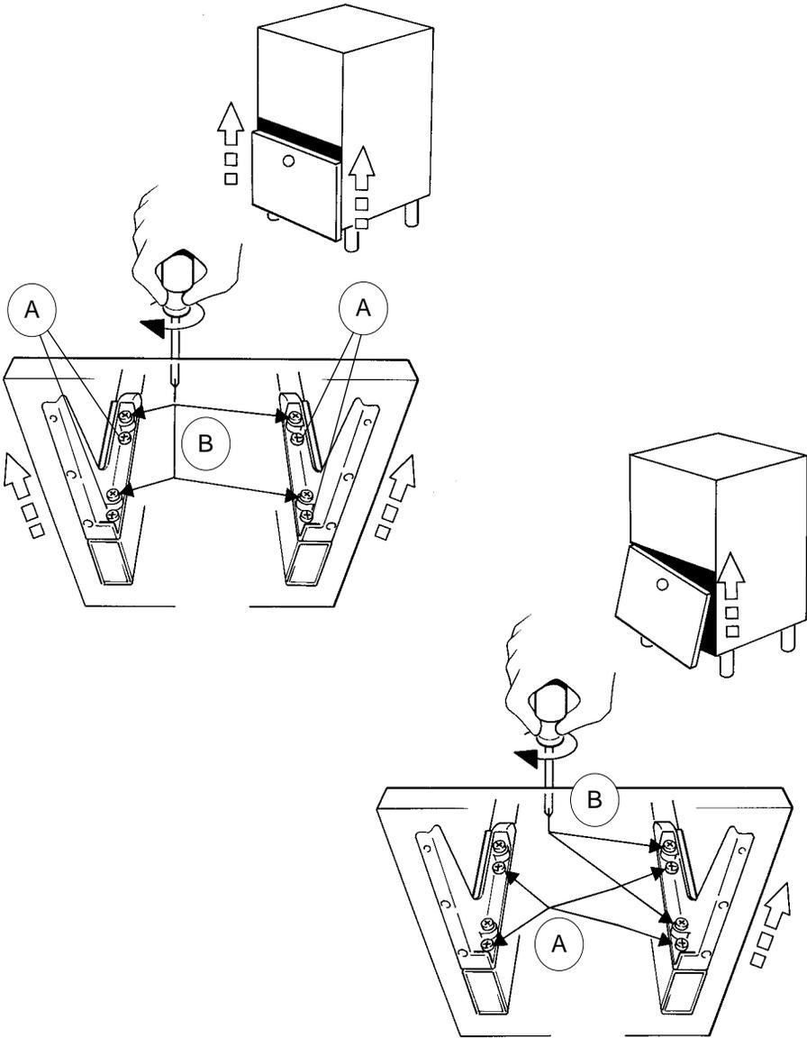
TO RAISE DOOR, LOOSEN ATTACHMENT SCREWS (A) AND TIGHTEN ADJUSTMENT SCREWS (B). TO LEVEL DOOR, RAISE LOW SIDE ONLY UNTIL DOOR IS LEVEL.
