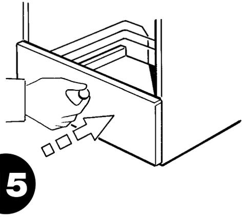
WITH SLIDES IN CLOSED POSITION, SET UNIT ON SLIDES AND PUSH IN AS FAR AS IT WILL GO. THIS WILL ENGAGE LOCK ON TO SLIDES.
