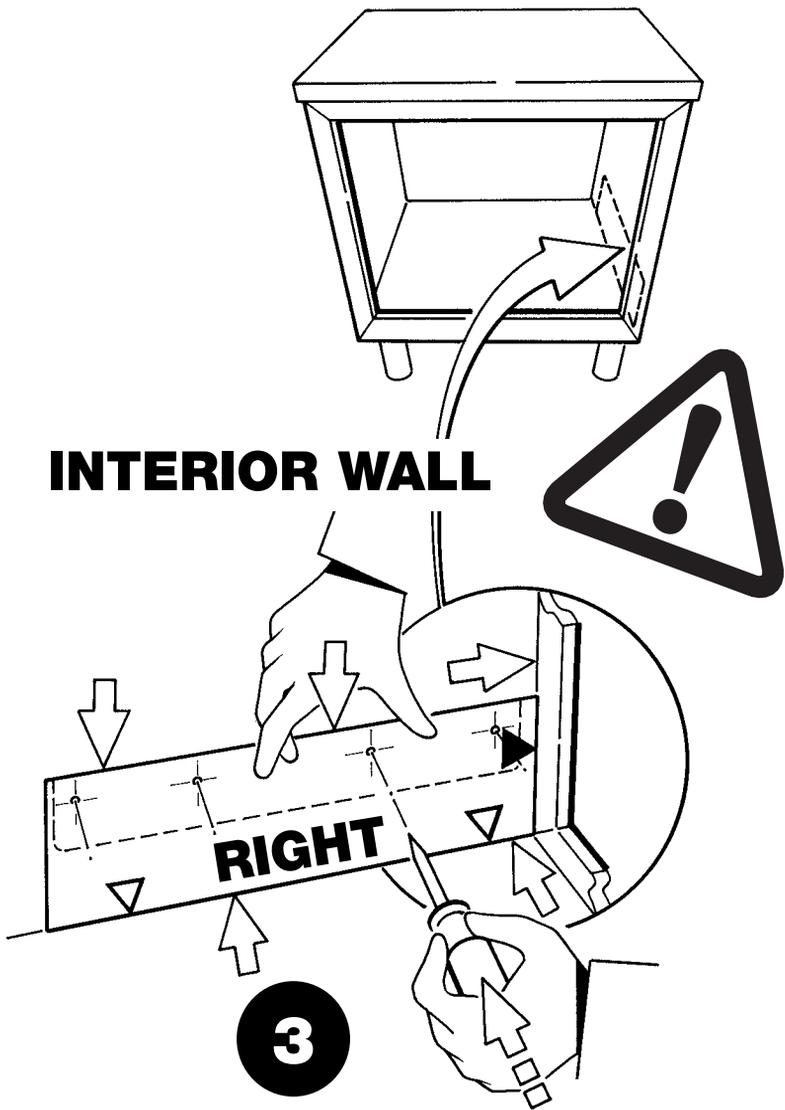
DRILL PILOT HOLES IN EACH SIDE OF CABINET AT LOCATION FOUND BY THE TEMPLATE
