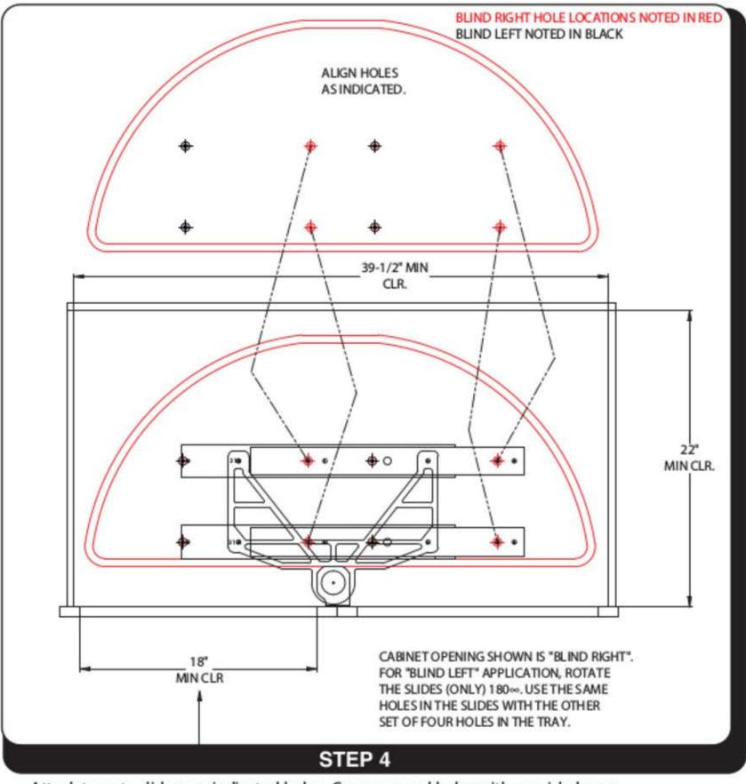
Attach trays to slides per indicated holes. Cover unused holes with provided caps.
