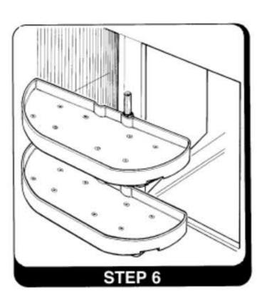
Now slide the pivot & slide assembly on shaft so it rests on the top postioner base. Your installation is now complete and should look like the illustration.
