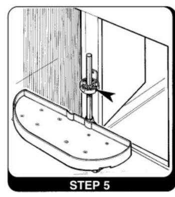
Take your pivot & slide assembly, match it over the bottom positioner base and insert the shaft through the top positioner base until the shaft bottom (open end) sets on cabinet bottom. Now tighten the set screws on both positioner bases (arrow points out top set screw). Be sure to tighten bottom positioner base set screw (not visible).
