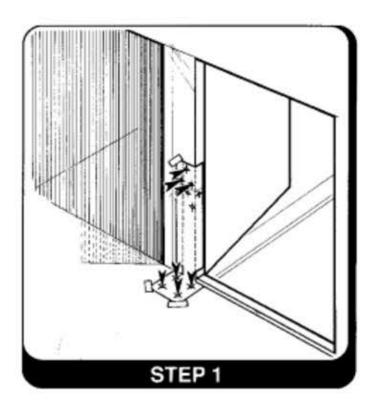
Position and tape template on inside of the face frame vertically (hinge side) as show in illustration. Using a 1/16" diameter bit, drill 5/8" deep pilot holes through the template at the 7 arrow locations. NOTE: Be careful not to drill through the front of the cabinet frame.
