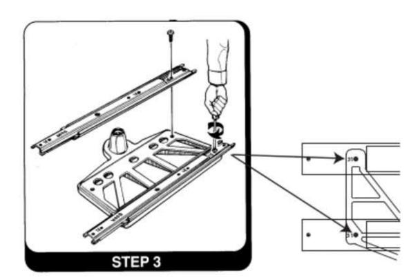
Attach slides to support frame starting with the hole location noted "31" (see illustrations. **NOTE:** Place end noted "this end away from cabinet opening" **AWAY** from cabinet opening. This will ensure proper function and alignment with other hole location.
