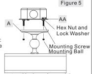
unscrewing the preassembled hex nut and lock washer and then screwing the mounting screws in or out of the crossbar until the correct length is achieved. Once the Ceiling Canopy (A) is secure, remove the mounting ball and Ceiling Canopy (A) and proceed to Step 6.
