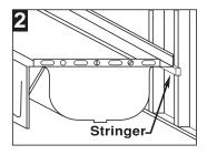
2. Tack the 2" x 4" stringer at a height that allows the tub to sit level, resting on the foam support pad. The stringer must run the full length of the tub. INSTALL-ING THE TUB WITHOUT A FULL LENGTH SUPPORT STRINGER WILL VOID THE WARRANTY.
