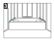
3. Check level in all directions. Use wood shimming if necessary. DO NOT shim under styrofoam support pad, it is required that the foam support pad rest on the floor. The floor should be flat and level. Once tub is level permanently fasten stringer to the studs. DO NOT fasten through tub flange.
