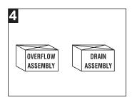
4. Install drain & overflow assemblies as directed by the manufactuerer. DO NOT over tighten the fittings connected to the tub. OVER TIGHTENING THE DRAIN CAN DAMAGE THE TUB AND VOID THE WARRANTY.
