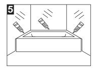
5. Install wall material & seal along wall-tub area using a bead of caulking or silicon resulting in a watertight joint.
