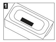
1. When removing tub from carton do not remove pad from tub bottom, removal voids warranty. Pads and blankets should be used to prevent damage. DO NOT STAND on the top of the tub.
