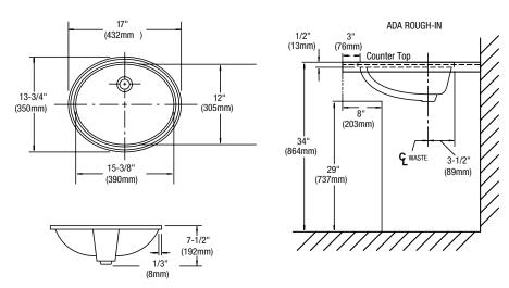
\*All dimensions and specifications are nominal and may vary: Dimensions of 8" and greater have a tolerance of +3%. Dimensions less than 8" have a tolerance of +5% Please utilize the current cutout template for countertop cutouts.
