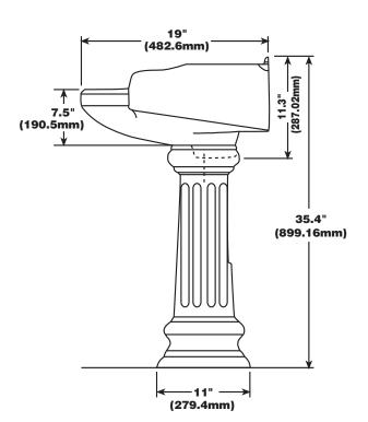
Note: All dimensions and specifications are nominal and may vary: Dimensions of 8" and greater have a tolerance of +3%. Dimensions less than 8" have a tolerance of +5%.
