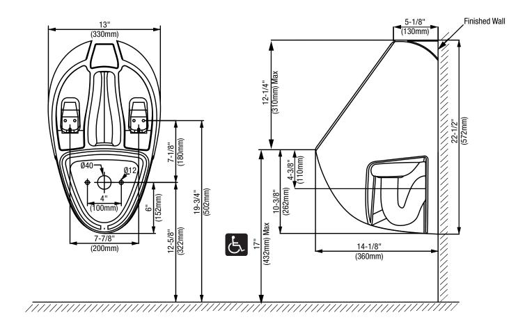
All dimensions and specifications are nominal and may vary: Dimensions of 8" and greater have a tolerances of +3%. Dimensions less than 8" have a tolerances of +5%.
