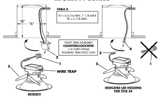
Fits into Prescolite 6" recessed cans including: DBX, RMNICD, IBXHW, FT6. Fits into most competitive recessed cans with "A" and "B" dimensions above including: Halo H7ICAT, H7RICAT; Juno IC22; Lithonia L7X; Capri CR1, CRR1; Progress P87-AT, P87-ATQC, P187-TG, P821-FB; Nora NHIC-17QAT, NHRIC-17QNBAT; Sea Gull 1128. See www.prescolite.com for more details.
