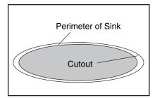
After checking fit and alignment of sink to cut out, apply a bead of silicone adhesive to rim of sink. The use other compounds is not recommended.
