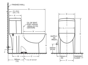
Hydraulic performance, water surface area, trap seal depth, ballpass diameter, and all fixture dimensions meet or exceed ANSI Standard A112.19.2M requirements.
