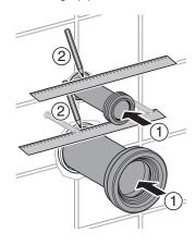
Place discharge pipe with gasket into waste outlet of bowl.
