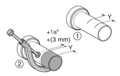
Remove protective sleeves from mounting rods. Determine protruding rod length for bowl installation. Install both pipes into the hubs in the wall.
