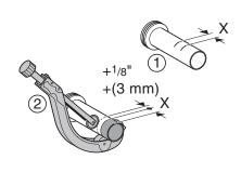
Add dimension Y and 1/8". Using that dimension, mark a line on the pipe measuring from the hub side. Cut off the pipe at the line with a pipe cutter.
