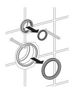
Insert discharge pipe into the pipe hub in the wall. Place a straight edge flush against the wall and mark a line on the pipe. Fit finned rubber seal onto flush pipe. Repeat same procedure for discharge pipe.
