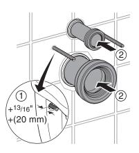
Bevel the sharp edges as shown to assure a smooth insertion into the pipe hubs in the wall.
