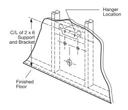
If molding is present and prevents installation of the vanity flush against the wall, notch the molding and/or provide suitable spacer for a secure installation.
