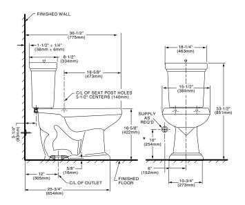
Hydraulic performance, water surface area, trap seal depth, ballpass diameter, and all fixture dimensions meet or exceed ANSI Standard A112.19.2M requirements.
