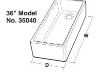
**D:** 17-7/8" TO 18-3/8" (454 to 466mm) **W:** 35-3/4" TO 36-1/4" (908 to 920mm)
