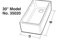
**D:** 17-7/8" TO 18-3/8" (454 to 466mm) **W:** 29-3/4" TO 30-1/4" (756 to 768mm)
