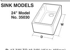
**D:** 17-7/8" TO 18-3/8" (454 to 466mm) **W:** 23-3/4" TO 24-1/4" (604 to 616mm)
