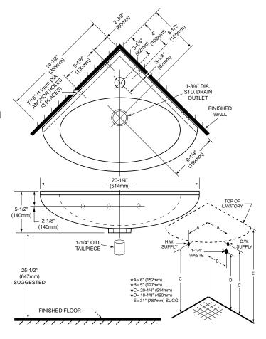
★ DIMENSIONS SHOWN FOR LOCATION OF SUPPLIES AND "P" TRAP ARE SUGGESTED. PROVIDE SUITABLE REINFORCEMENT FOR ALL WALL SUPPORTS.
