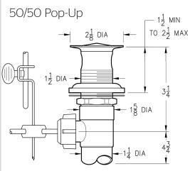
Ø1 Min to Ø1-1/2 Max. Deck Hole Openings
