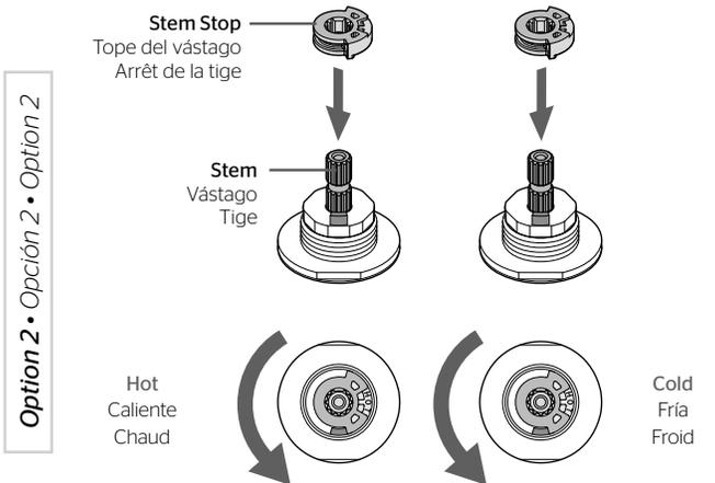
Stem Stop can be inserted into Stem in either of two ways, depending on the rotation you want to have for your handles.
