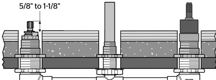
**!** Pfister™ Stem Extension Kit 974-375 must be used. Sold separately. Trim will not work if the stem height is less than 5/8" and more than 1-1/8".
