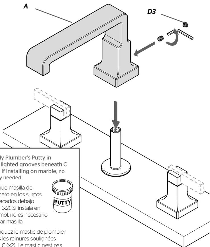
Apply Plumber's Putty in highlighted grooves beneath C (x2). If installing on marble, no putty needed.
