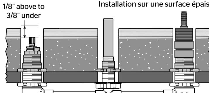
**!** Two Pfister™ 974-375 Stem Extension Kits must be used. Sold separately. Trim will not work if stem is located more than 3/8" below the deck and more than 1/8" over the deck.
