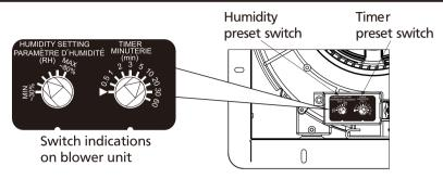
Humidity preset switch positions (Tolerance:±10%)
