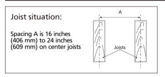
If the spacing A is 16 inches (406 mm) to 24 inches (609 mm) on center joists, please follow the installation step as below.
