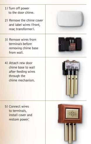
\*When upgrading from a 2-note chime to a NuTone 4 or 8-note chime, it will be necessary to add two nine-volt batteries.
