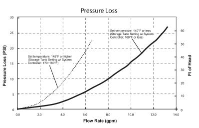
**NOTE:** For Quick-Connect and Multi-System installations, pressure loss remains constant throughout the system regardless of the number of units installed. Multiply the total number of units in the system by the required flow rate from each unit to determine the total pressure loss from the chart above.
