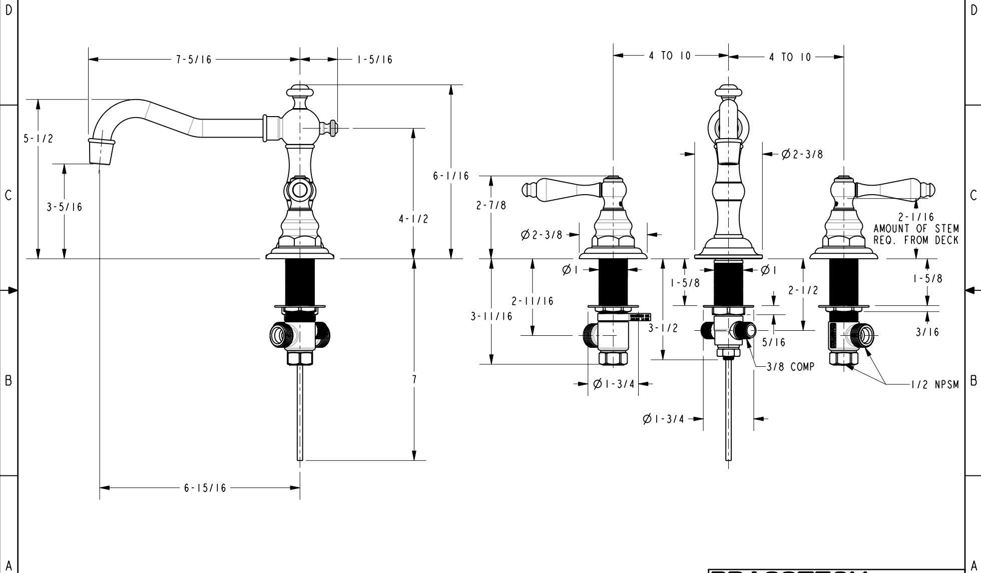
DIMENSIONS ARE IN INCHES AND AN APPROXIMATION OF A TYPICAL INSTALLATION
