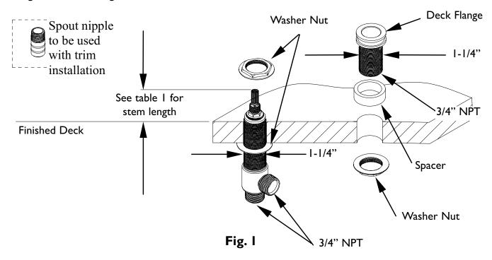
3. Attach hot/cold valves to spout, utilizing 3/4" copper pipe. See Figure 2.
