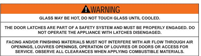
BEFORE DOOR IS REMOVED TURN THE APPLIANCE OFF AND WAIT UNTIL APPLIANCE IS COOL TO THE TOUCH. DOORS ARE HEAVY AND FRAGILE SO HANDLE WITH CARE.
