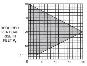
HORIZONTAL VENT RUN PLUS OFFSET IN FEET  $H_{\tau}$ The shaded area within the lines represents acceptable values for  $H_{\tau}$  and  $V_{\tau}$
