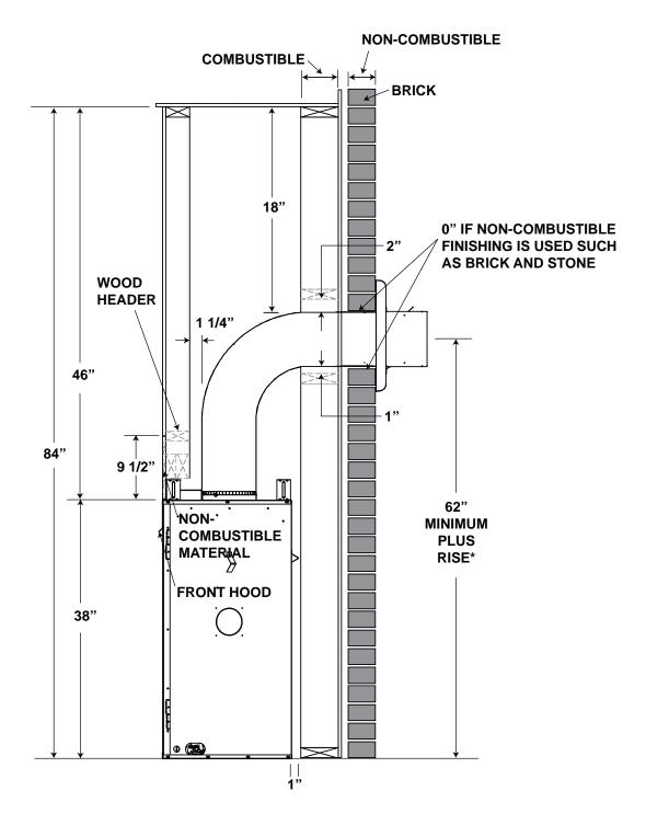
For temperature requirements, the enclosure space around and above the appliance must be left unobstructed. It is recommended that the enclosure be ventilated at the top and bottom to circulate the hot air.
