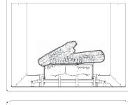
**6.2.5** Align the holes in the bottom of the right log (W135-0447) with the pins in the rear and front right log.
