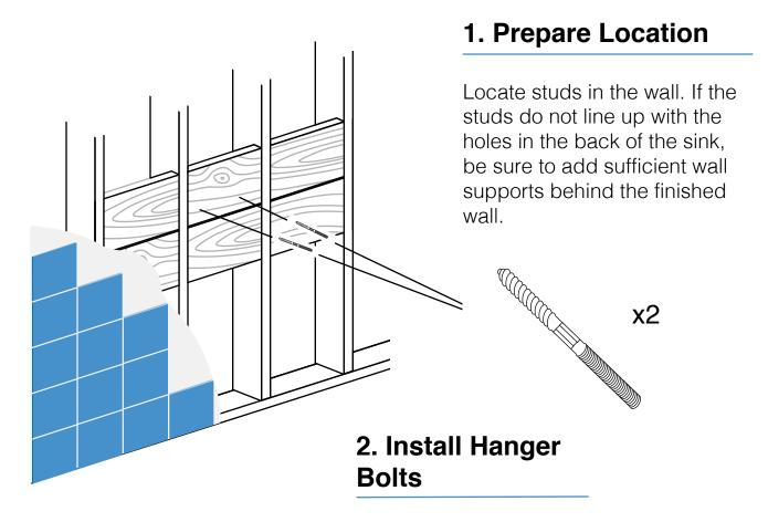
Measure the distance between mounting holes in the back of the sink. Drill pilot holes in wood and screw in hanger bolts. Check position with a level.
