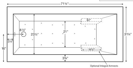
The Sculpted Finish process does not allow enough space for mounting fixtures on the tub deck. Shown as Air Bath
