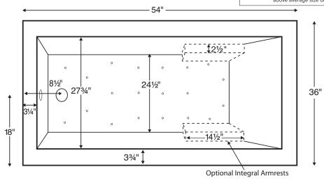
The Sculpted Finish process does not allow enough space for mounting fixtures on the tub deck. Shown as Air Bath
