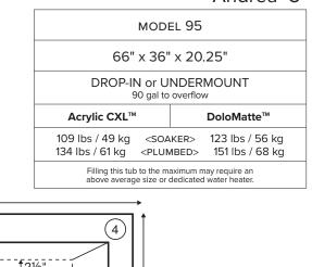
66! 3 0 \$21/2 0% 0) 283% · 26<sup>1</sup>/4" 36' 81/2 10 Compliance Label Model MTXXXX 18 Made in USA 0 Complies with ANSI 2124.1-1995 CSA Certified C/US 2 1 31⁄2" Numbered areas on tub deck represent possible locations to install cleaning systems, faucets and other fixtures. Shown with Air Massage and Ultra Whirlpool Package. 58' 122 20'1/4" 191/2" 181/2 171/2 103
