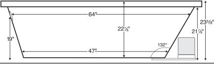
IMPORTANT: Air baths and tubs with a pre-leveled foam base or frame system add 2-3" to overall tub height.
