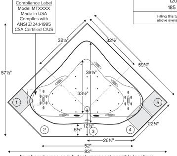
Numbered areas on tub deck represent possible locations to install cleaning systems, faucets and other fixtures.
